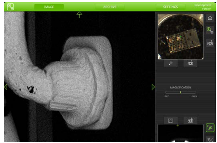
The Phenom XL user interface with a tilted sample. The meta data of all saved images include all relevant tilt and rotation angles.
